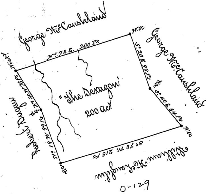
A Draught of a survey call'd "The Hexagon" situate situate on the Waters of Kings Creek in Washington County, containing 200 ac<sup>ts</sup> and the Allow<sup>ce</sup> executed Sep<sup>r</sup> 2<sup>d</sup> 1789 in Pursuance of a Warrant granted to W<sup>m</sup> Braden for 200 ac<sup>ts</sup> dated Novemb<sup>r</sup> 21<sup>st</sup> 1788.
